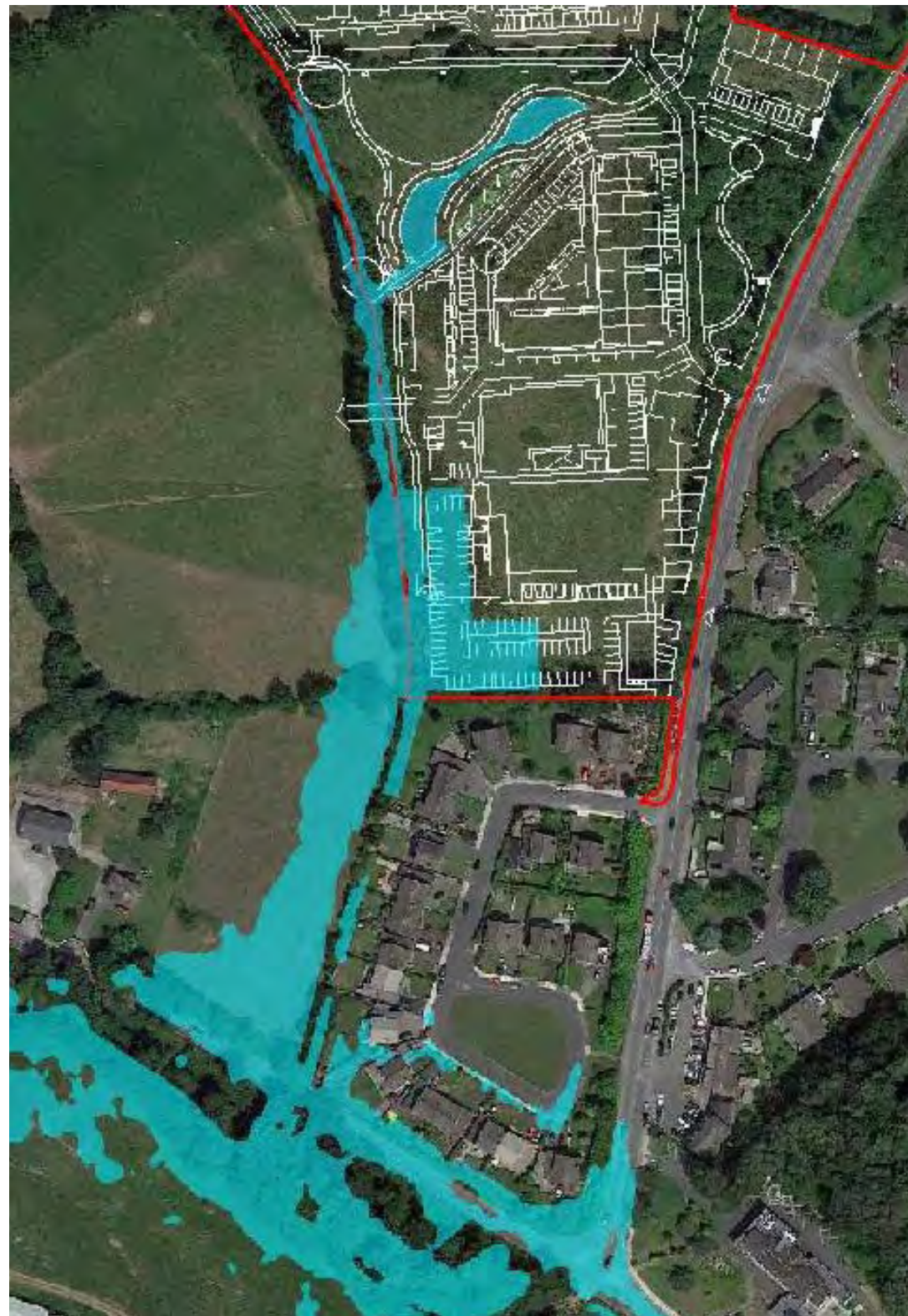
Figure 8.19c: Flood mapping, developed terrain, stream flow = 0.1% AEPCC (2.2m 3 /s), river flow = 10m 3 /s
