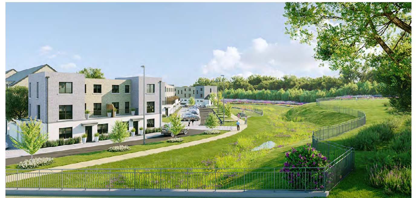
Figure 4.5c – Visualisation of the central amenity and attenuation area. Seeded with native wildflower species for damp meadows and planted with plugs of Rush and Flag Iris for biodiversity and water filtration.
