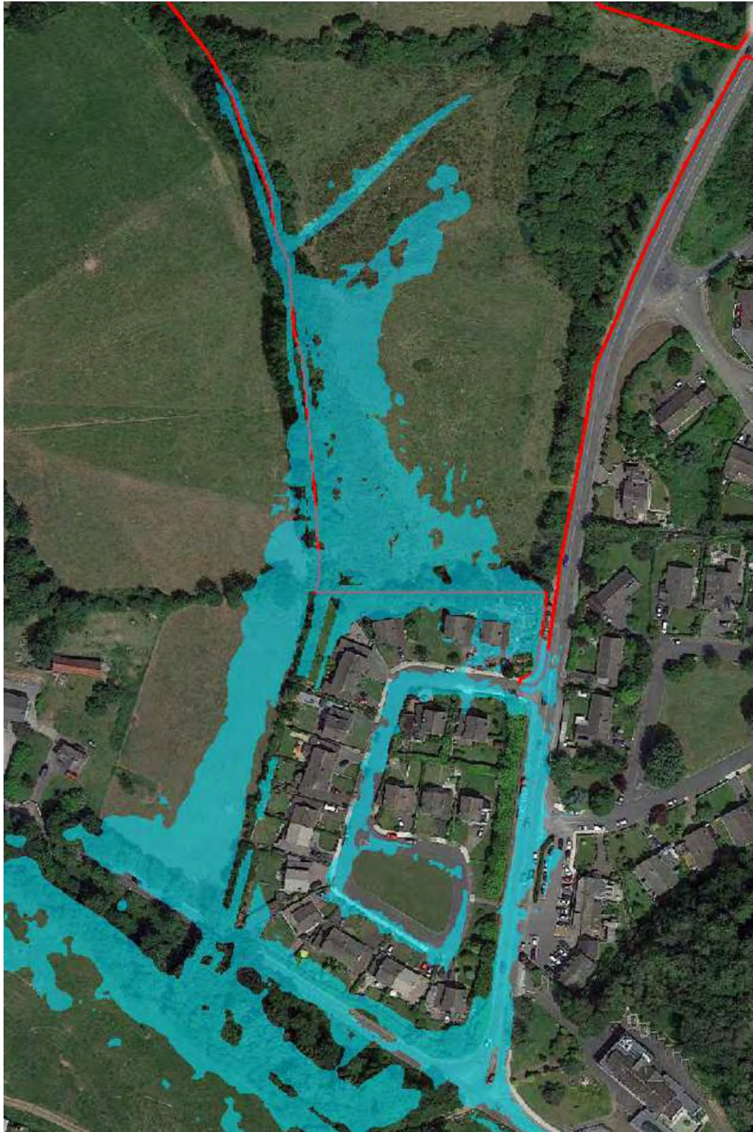
Figure 8.13b: Flood mapping, existing site terrain, stream flow = 1%AEPCC (1.7m 3 /s), river flow = 10m 3 /s
