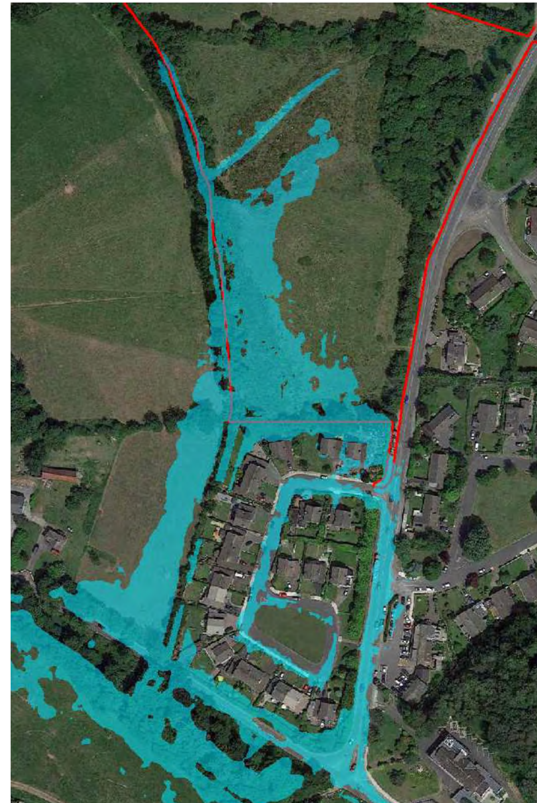
Figure 8.13a: Flood mapping, existing site terrain, stream flow = 1%AEP ( 1.4\text{m}^3/\text{s} ), river flow = 10\text{m}^3/\text{s}
