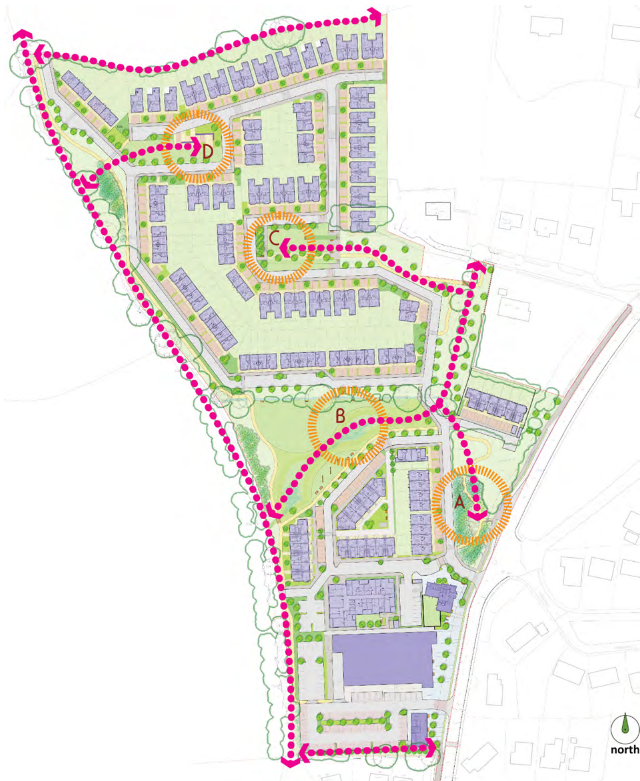
Figure 4.5b – Diagram of biodiversity links overlaid onto the Landscape Masterplan. The pink dashed lines indicate contiguous tree planting and habitat corridors, with the aim of linking back to the stream along the western boundary. Four primary biodiversity zones (A-D) are highlighted.
