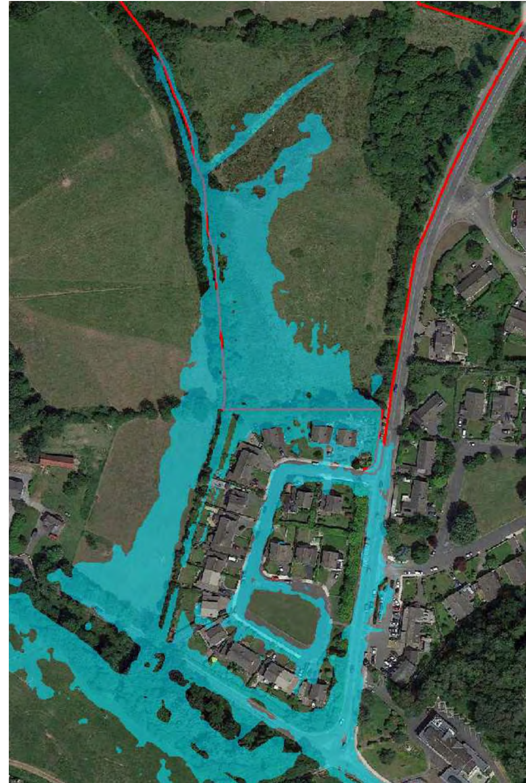
Figure 8.13c: Flood mapping, existing site terrain, stream flow = 0.1%AEPCC (2.2m 3 /s), river flow = 10m 3 /s
