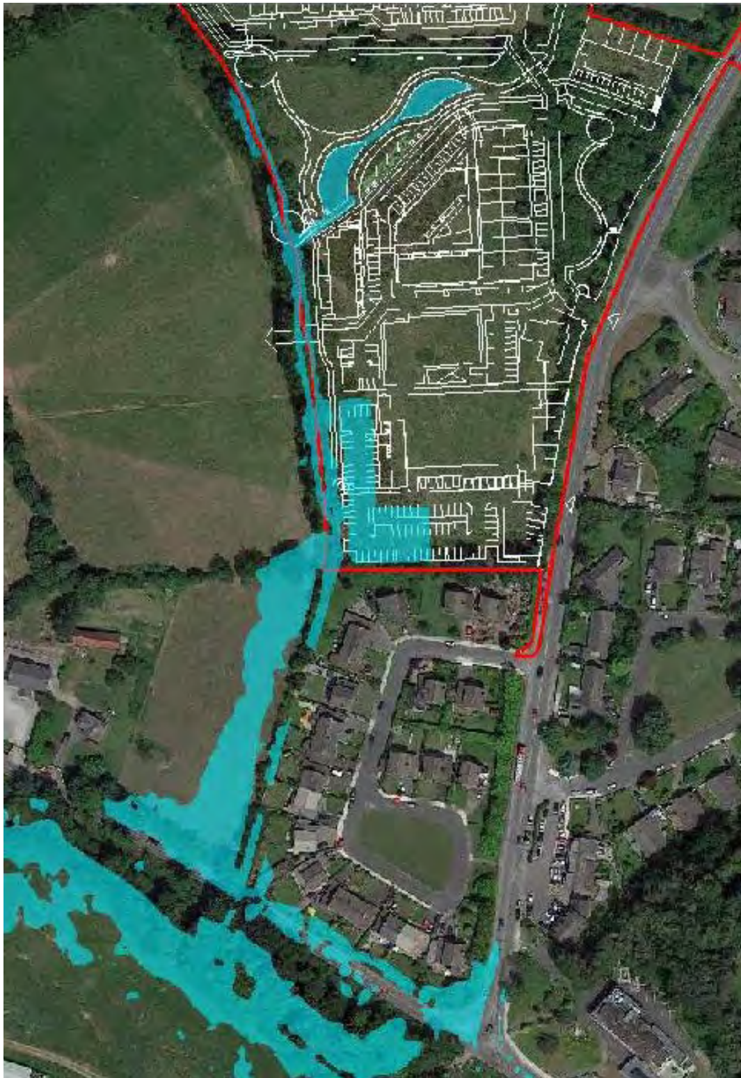
Figure 8.19a: Flood mapping, developed terrain, stream flow = 1%AEP (1.4m 3 /s), river flow = 10m 3 /s
