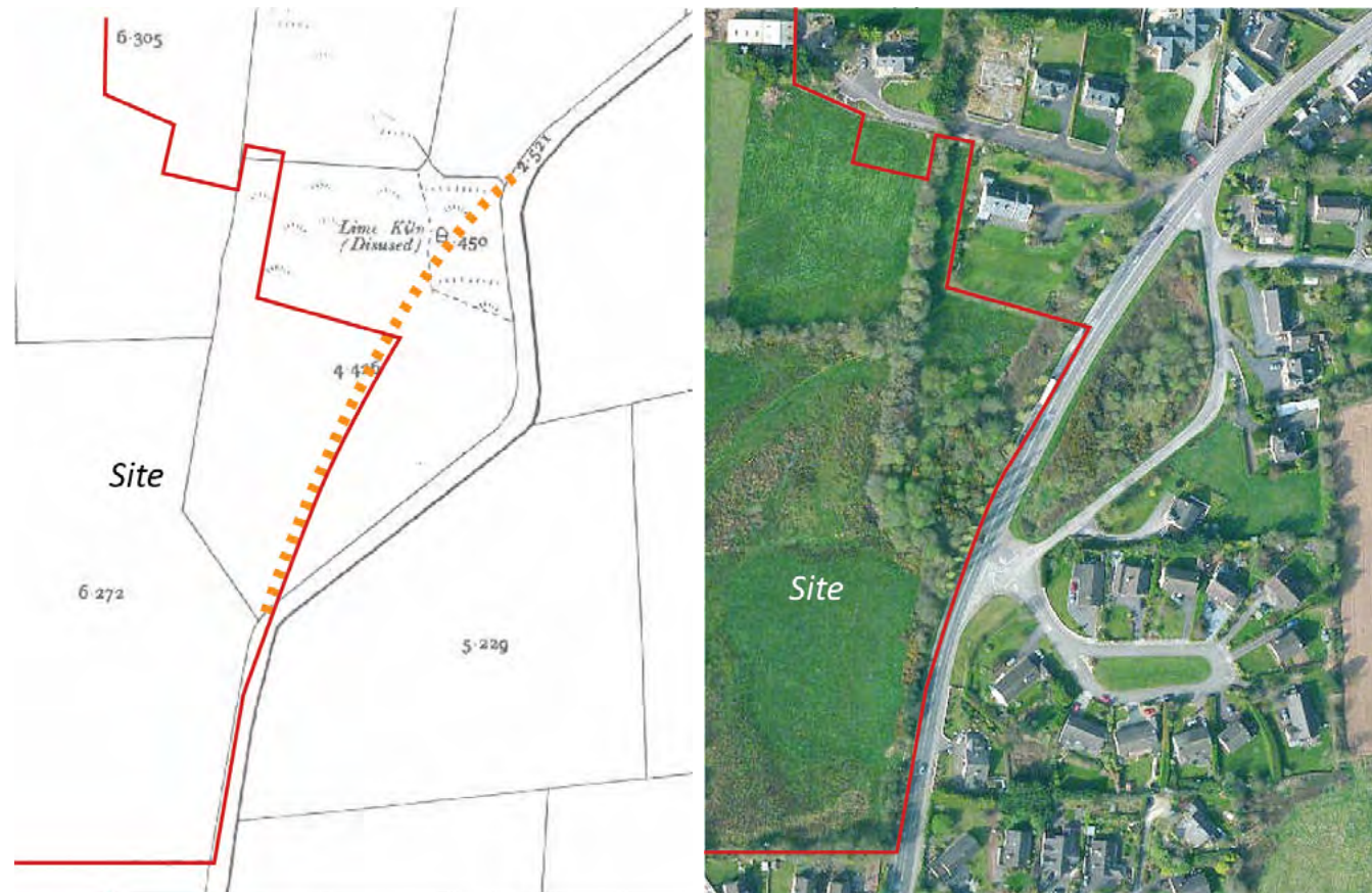
Figure 4.4a – Image of 25-inch map (early 1900’s) illustrating the original route of the current R617 (dashed orange line). The diversion would most likely have been circumventing a valley or recess in the terrain. (bottom) Aerial image showing the new R617 road with the old road still in existence.
