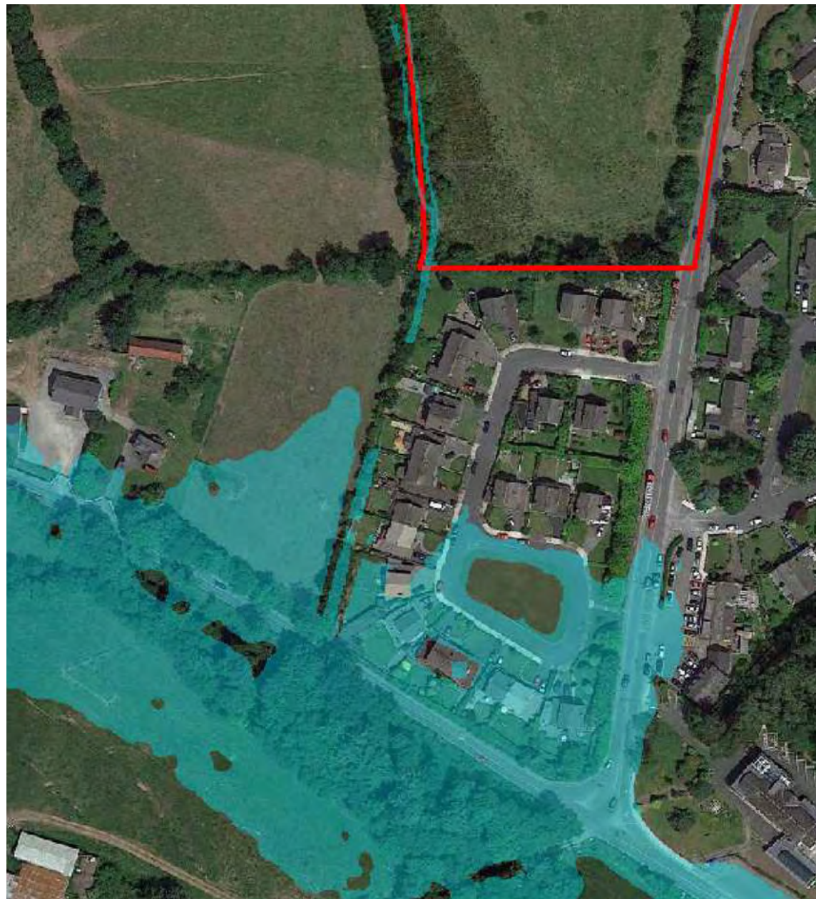
Figure 8.12: Extent of inundation arising from 1%AEPCC ( 44\text{m}^3/\text{s} ) peak flow in the river and a nominal flow in the western stream ( 0.2\text{m}^3/\text{s} )
